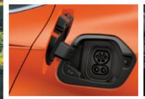
CHARGING OPTIONS Quick and easy: charge your Corsa-e battery up to 80 % in 30 minutes<sup>2</sup> only, at specifically designed wall boxes, public charging stations or regular home sockets.
