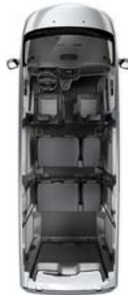
8-seater with 2 single seats in the front, 2-seater bench and 1 single seat in the second and third row, pulled down.
