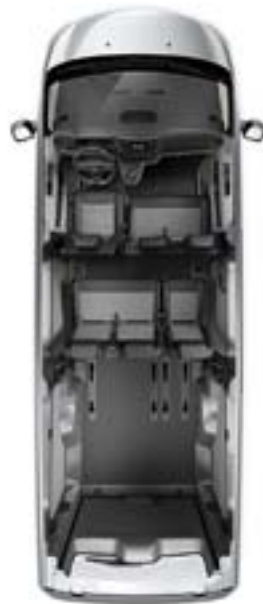
6-seater with 1 single seat and 2-seater bench in the front and in the second row.
