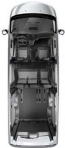
5-seater with 2 single seats in the front and 2-seater bench and 1 single seat in the second row.
