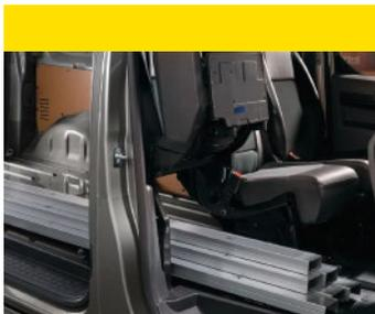
**Cabin:** fold the base of the outer front passenger seat up against the seat back to load bulky cargo such as large boxes into the front of the van.<sup>1</sup>
