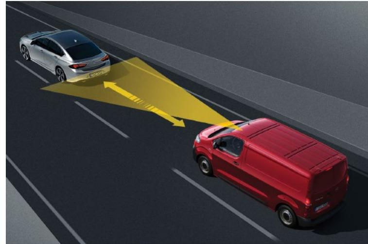
**Forward Collision Alert<sup>1</sup>:** scans the road ahead to alert the driver to the potential for a collision with vehicles or pedestrians. Additionally, the **Semi-adaptive Cruise Control<sup>1</sup>** lowers your speed to maintain a set distance to the car ahead in traffic scenarios and restores your previous speed when the road clears.
