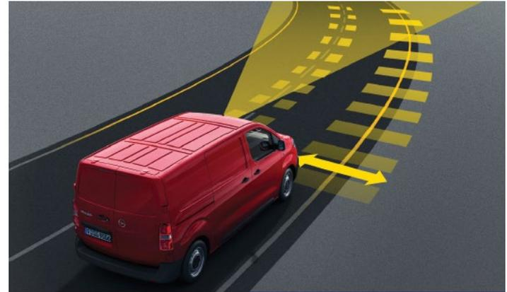
**Lane Departure Warning<sup>1</sup>:** recognizes when the Vivaro is drifting lanes and alerts the driver via audio and visual cue.
