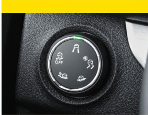
**IntelliGrip<sup>1</sup>:** the Vivaro's IntelliGrip system, including special construction site tyres, provides extra levels of traction on difficult surfaces such as mud, sand or snow.
