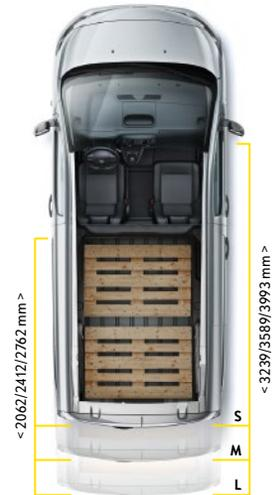
Available in 3 sizes of body length – Small, Medium and Large – the Vivaro perfectly adapts to your business needs, each variant offering a balance between relatively compact exterior dimensions and a spacious, flexible interior. The Small version in particular, at just 4,60 m in length, is perfectly agile in tight city streets and urban areas where space is limited. This variant can load 2 euro-pallets, while the Medium version can comfortably carry 3 euro-pallets.
