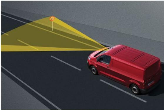
**Speed Limit Adaptation<sup>1</sup>:** uses Speed Sign Recognition to analyse changes in the speed limit. With one push of the memory button, allow Semi-adaptive Cruise Control to adjust your speed accordingly.
