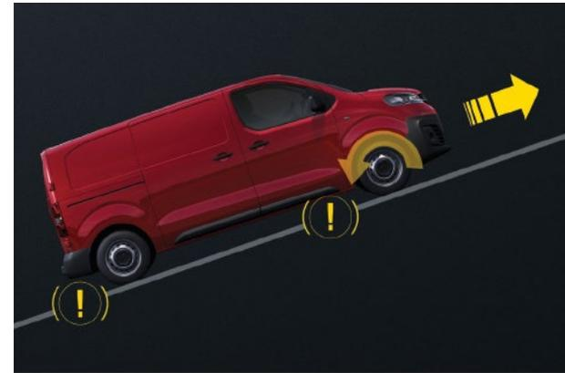
**Hill Climb Assist<sup>1</sup>**: keeps the car from rolling backwards when stopped on an incline and holds the brake for you while you switch from the brake pedal to the gas pedal. Once you operate the accelerator, it releases the brake.
