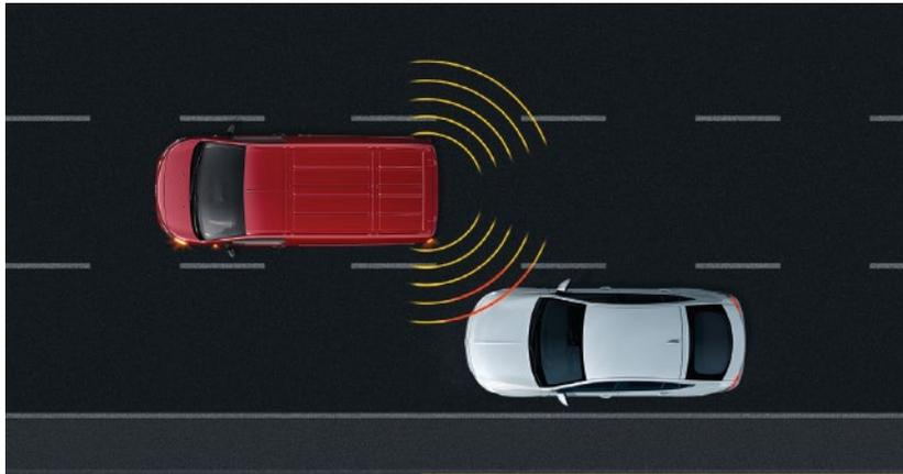
**Side Blind Spot Alert<sup>1</sup>**: uses sensors and a visual projection on the wing mirror, alerting the driver to vehicles in the Vivaro's blind spot to prevent accidents in overtaking situations.
